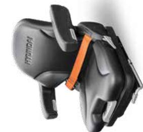
The high-quality Grammer seat features full suspension and an adjustable cushion to provide comfort for every driver. A seat belt switch, armrests and seat heating are available as options.
