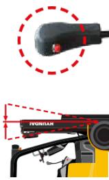
Auto tilt levelling ensures that the forks remain parallel to the ground. This enhances safety and work efficiency when loading and unloading pallets on and off high racks.
